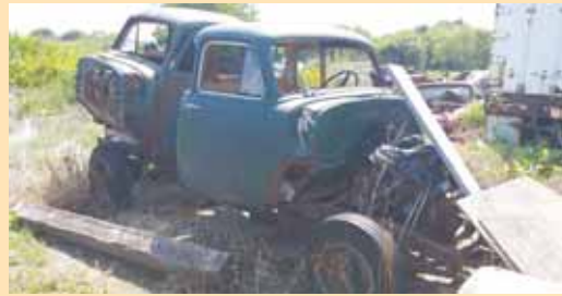
Plagemann found an old Chevy truck lying in the weeds and converted it into this "doodlebug". The front end, hood and grill are off an Oliver tractor.
