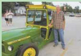
Robert Thomas wanted something unique for local parades so he built this stretched-out "Little Green Machine". It's fitted with a Hiniker cab and a Deere 5010 hood.
