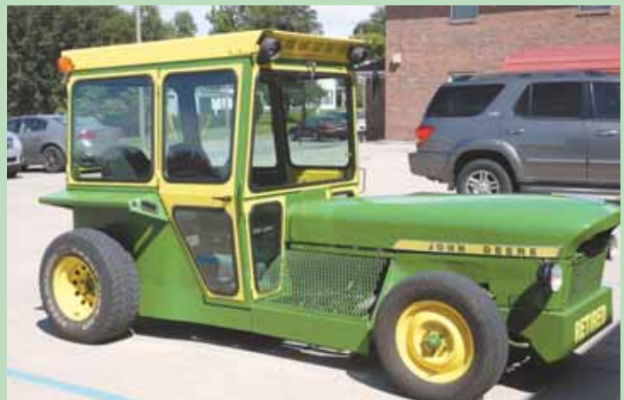
Robert Thomas wanted something unique for local parades so he built this stretched-out "Little Green Machine". It's fitted with a Hiniker cab and a Deere 5010 hood.
