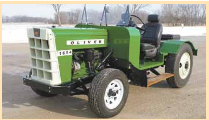
Plagemann found an old Chevy truck lying in the weeds and converted it into this "doodlebug". The front end, hood and grill are off an Oliver tractor.
