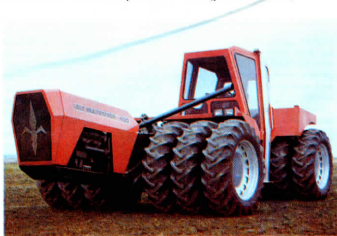
Two twin 210 hp engines power the new Lely Multipower 420. Rear engine can be used for pto drive, and the front engine to drive the tractor.
