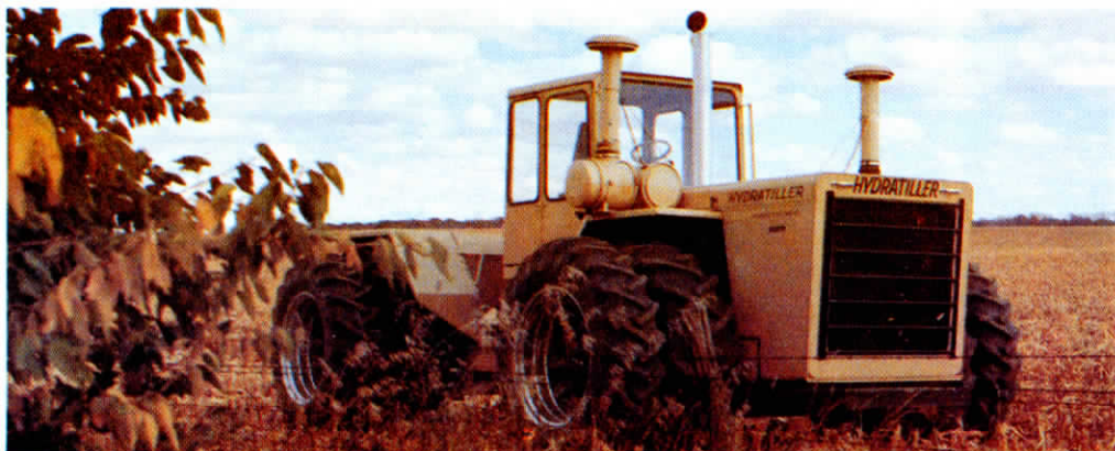
Each wheel of the revolutionary all-hydrostatic Hydratiller has its own drive motor.
